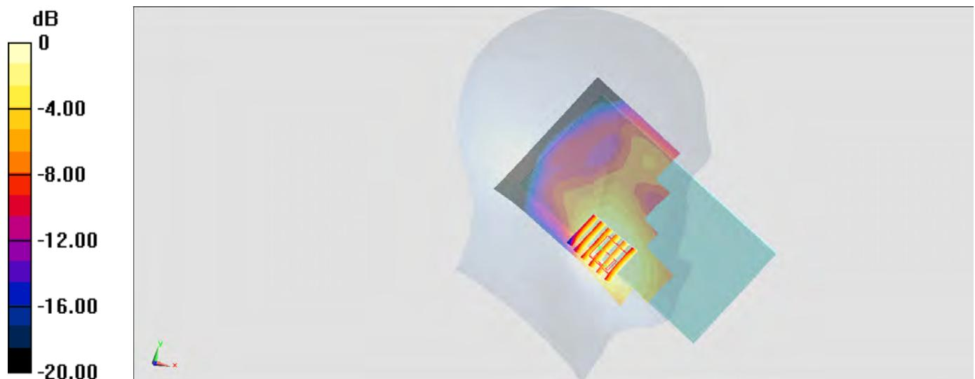
$$0 \text{ dB} = 0.115 \text{ W/kg} = -9.39 \text{ dBW/kg}$$
