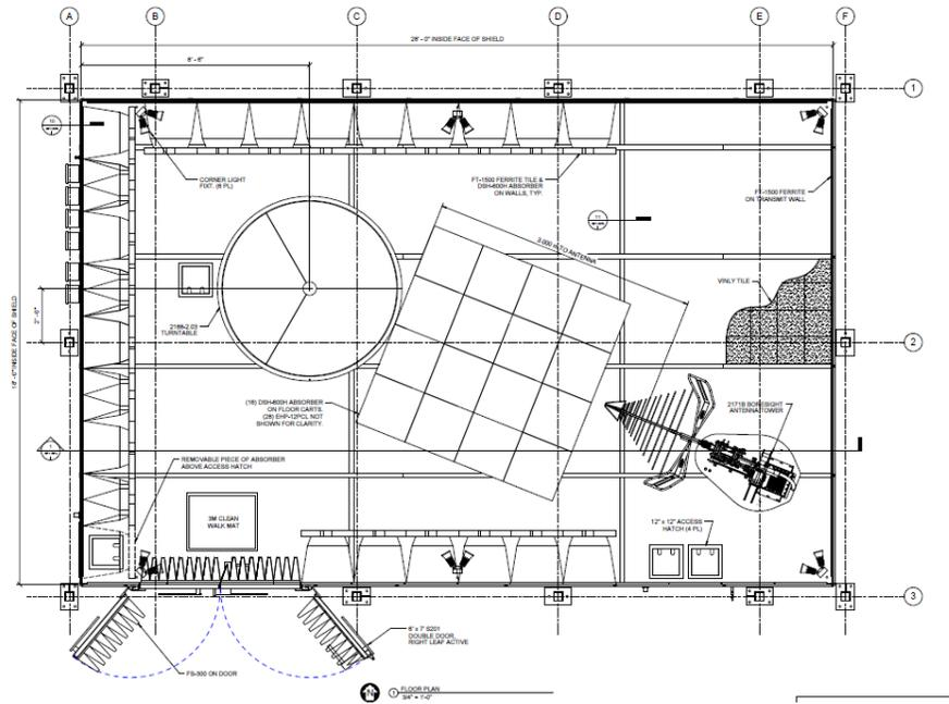
Figure 3. Radiated Emissions Disturbance Measurement Facility Diagram
