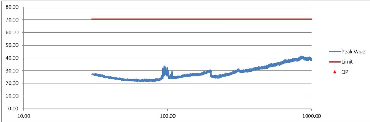
**Figure 10. Horizontal Antenna Position, 30-1000 MHz -Tamura Switching Power Supply**
