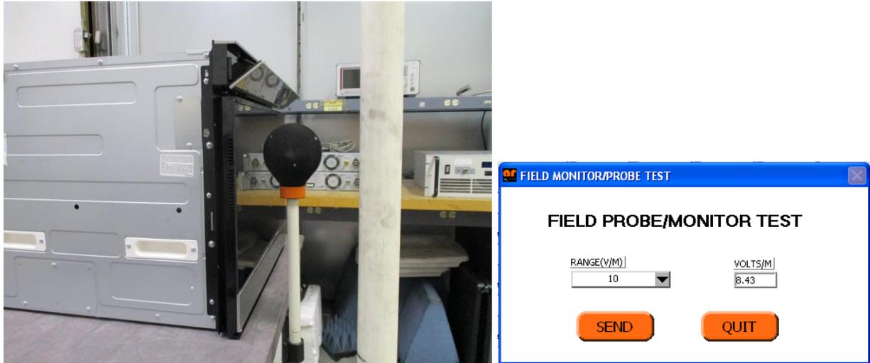
**Figure 23. Leakage from Tamura Switching Power Supply**
