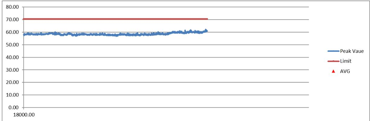
**Figure 8. Horizontal Antenna Position, 18 – 25 GHz - Mitsuoka Switching Power Supply**
