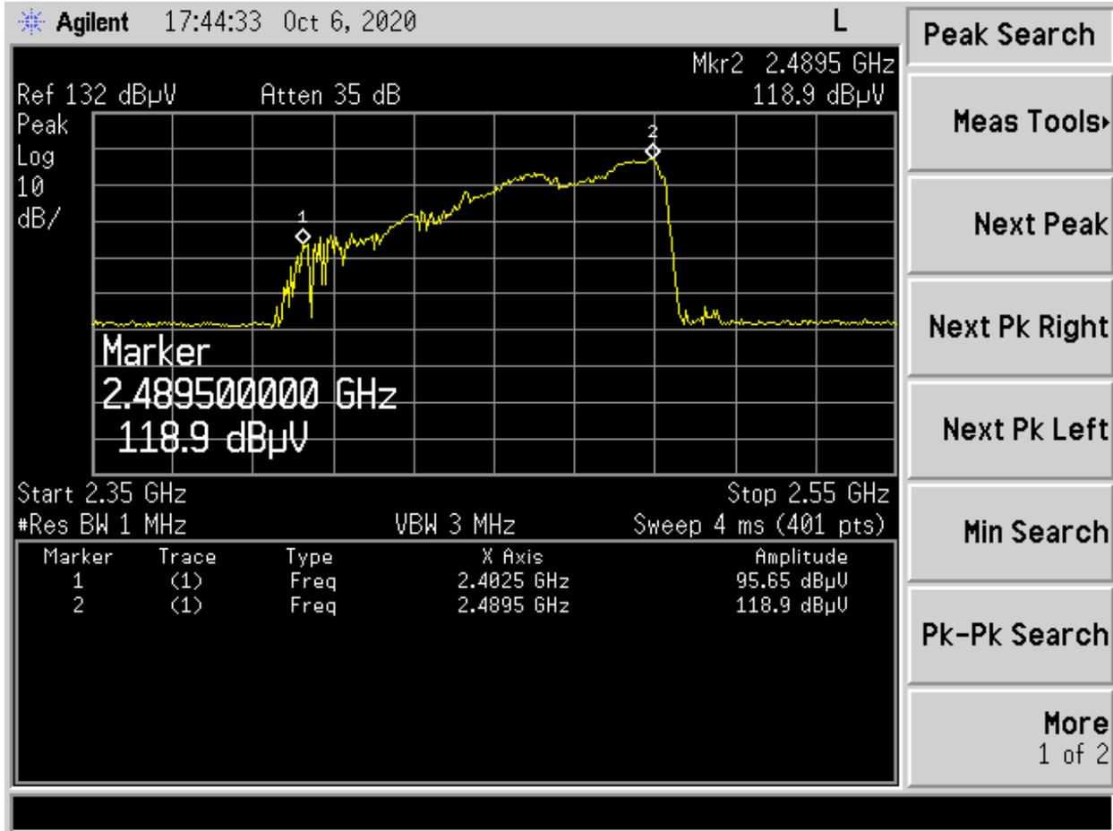
Figure 18. Frequency Variation at High Voltage - Mitsuoka Switching Power Supply
