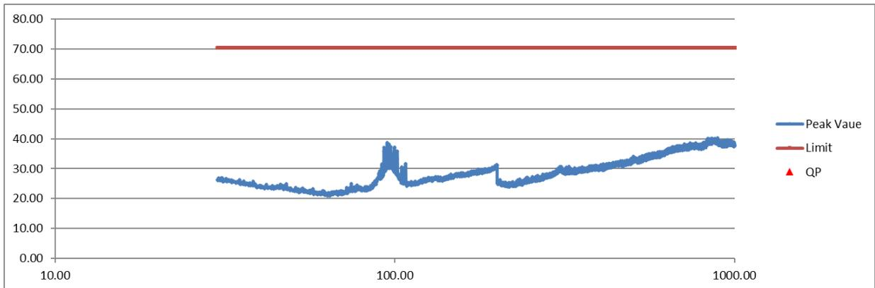
**Figure 11. Vertical Antenna Position, 30-1000 Mhz - Tamura Switching Power Supply**
