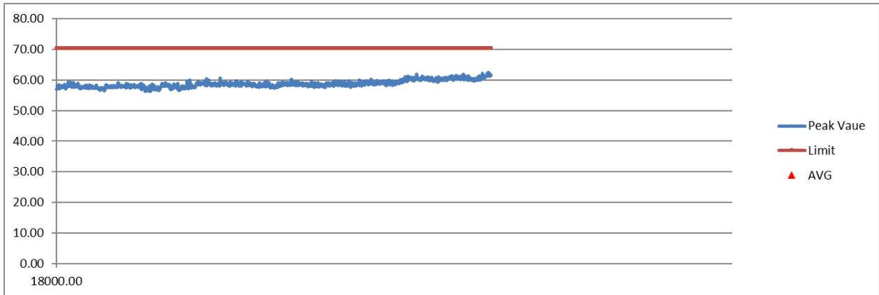
**Figure 9. Vertical Antenna Position, 18 – 25 GHz - Mitsuoka Switching Power Supply**
