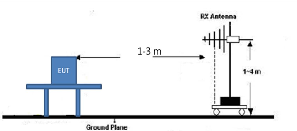
**Figure 1. Block Diagram of Radiated Emissions Test Configuration**
