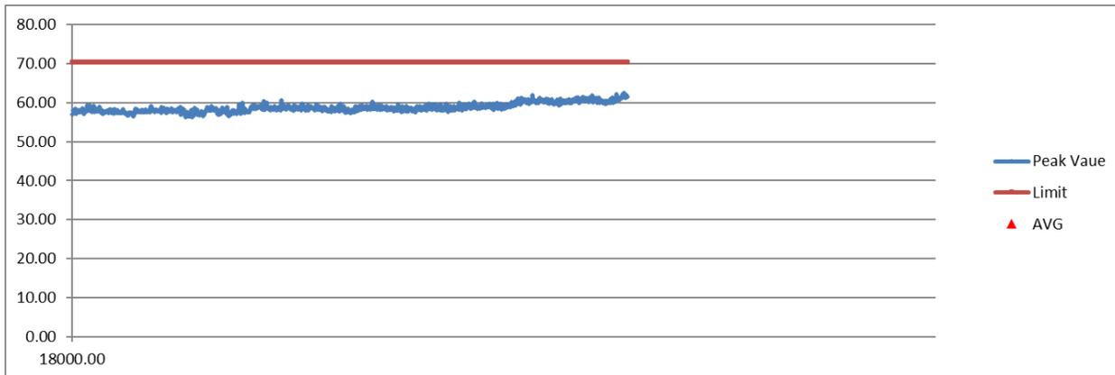
**Figure 15. Vertical Antenna Position, 18 – 25 Ghz - Tamura Switching Power Supply**
