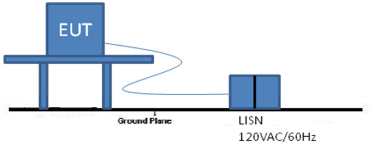
**Figure 2. Block Diagram of AC Power Lines Conducted Emissions Test Configuration**
