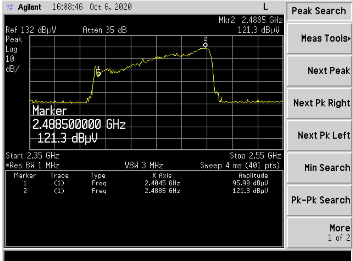
Figure 16. Frequency Variation at Nominal Voltage -Mitsuoka Switching Power Supply
