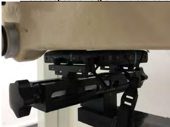
Fig.15 EUT Back side to flat phantom
