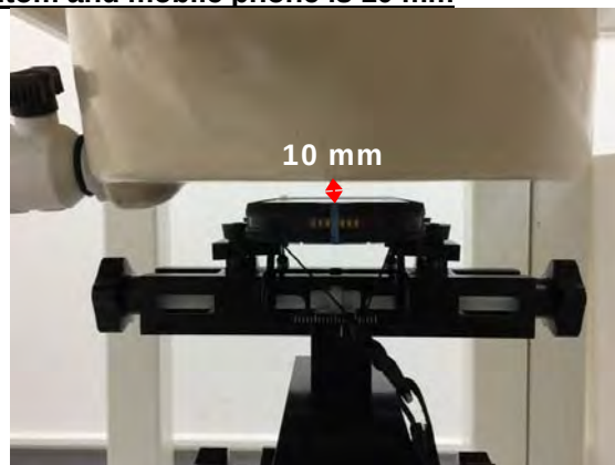
Fig.7 EUT Front side to flat phantom
