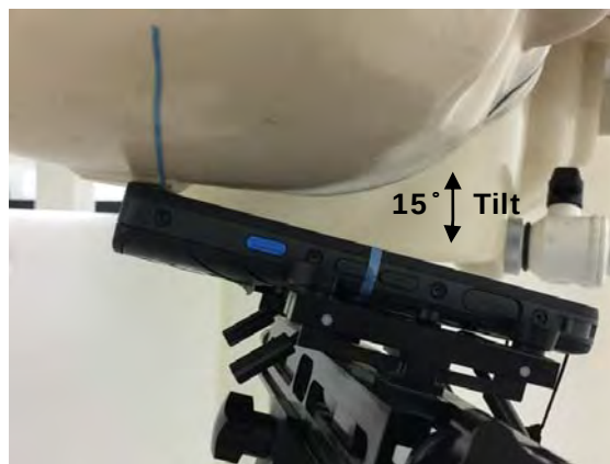
Fig.4 Right Head Section / Ear-Tilt Position(15°)
