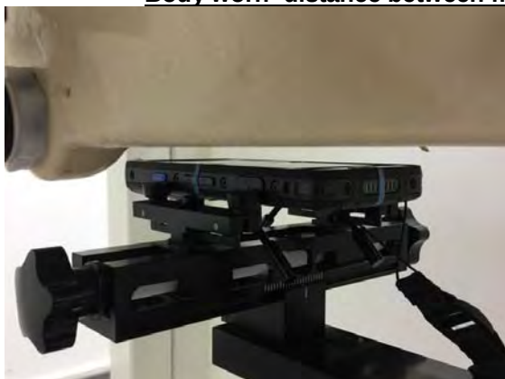
Fig.7 EUT Front side to flat phantom
