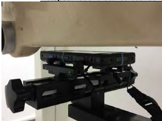
Fig.9 EUT Front side to flat phantom
