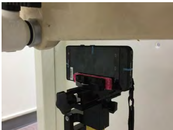
Fig.11 EUT Right side to flat phantom
