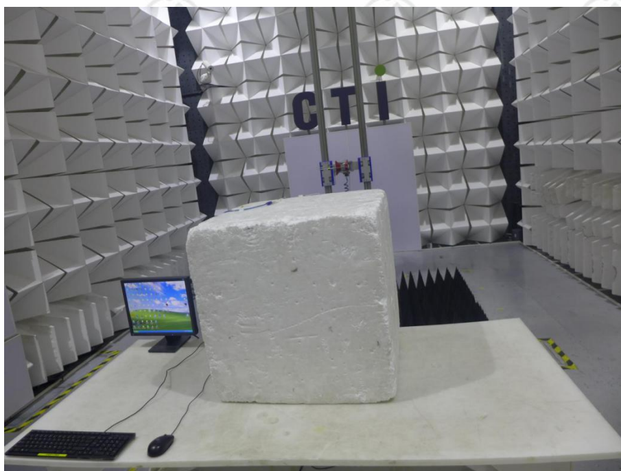
Radiated spurious emission Test Setup-3(Above 1GHz)
