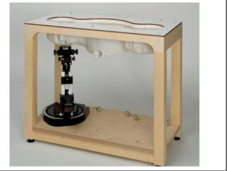
The bottom plate contains three pair of bolts for locking the device holder. The device holder positions are adjusted to the standard measurement positions in the three sections. A white cover is provided to tap the phantom during off-periods to prevent water evaporation and changes in the liquid parameters. On the phantom top, three reference markers are provided to identify the phantom position with respect to the robot.
