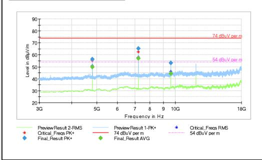
Note: According to FCC15.35(c), a duty cycle correction factor is applied here. Considering the limit of packets per interval and minimum interval of BTLE, this leads a correction factor of 17.86dB. Hence this margn could cover the highest spurious above.
