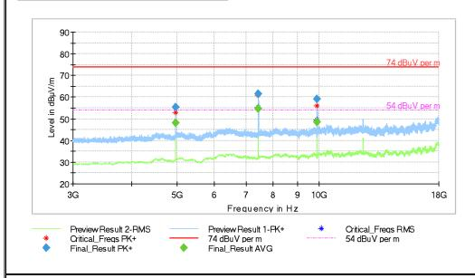
Note: According to FCC15.35(c), a duty cycle correction factor is applied here. Considering the limit of packets per interval and minimum interval of BTLE, this leads a correction factor of 17.86dB. Hence this margn could cover the highest spurious above.
