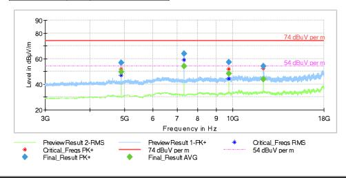
Note: According to FCC15.35(c), a duty cycle correction factor is applied here. Considering the limit of packets per interval and minimum interval of BTLE, this leads a correction factor of 17.86dB. Hence this margn could cover the highest spurious above.
