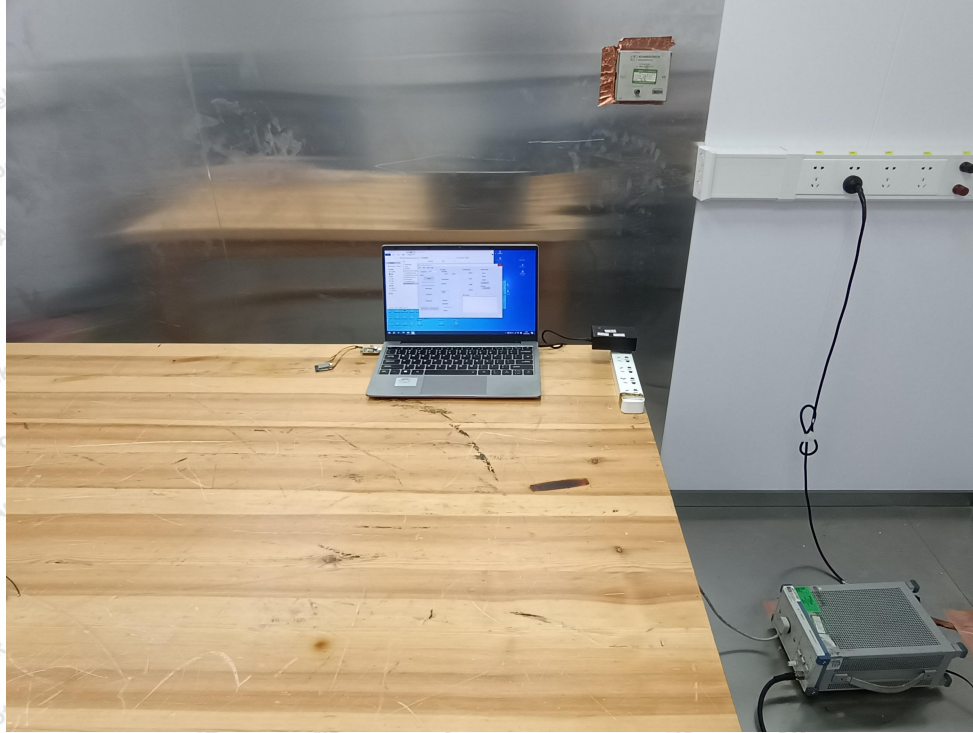
Photo of Conducted Emission Measurement
