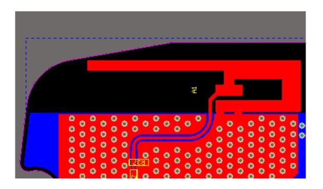
Inverted F Antenna designed in accordance with Texas Instruments Design Note DN00007
