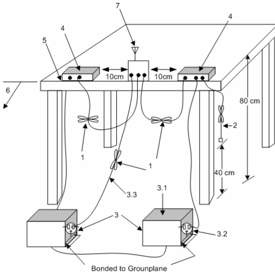
1. Interconnecting cables that hang closer than 40 cm to the ground plane shall be folded back and forth in the center forming a bundle 30 cm to 40 cm long see (see 6.2.3.2).
