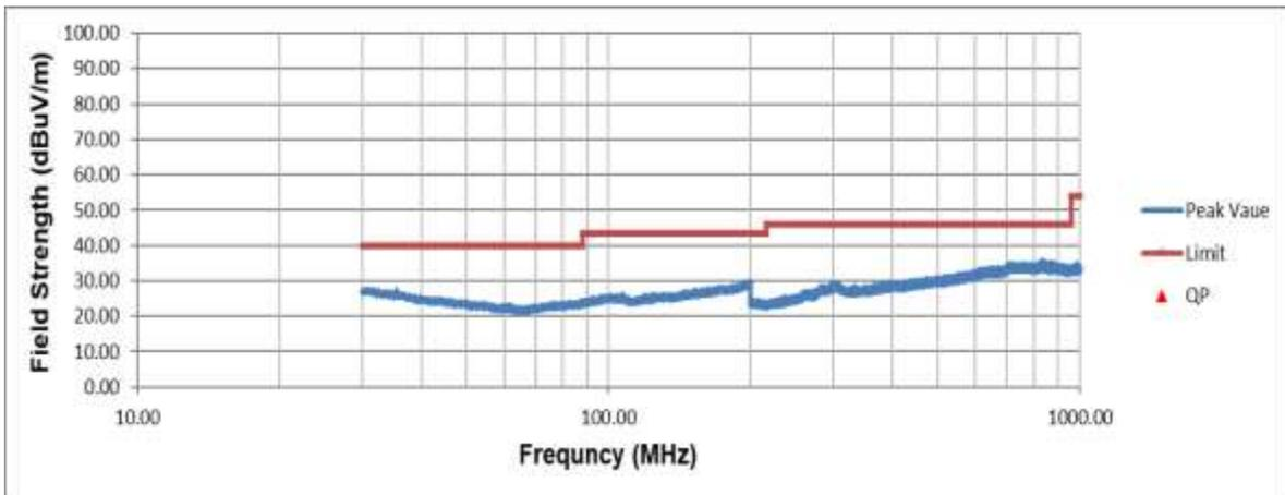
Figure 17. Unintentional Radiated Emissions, 30 MHz – 1000 MHz (Vertical)
