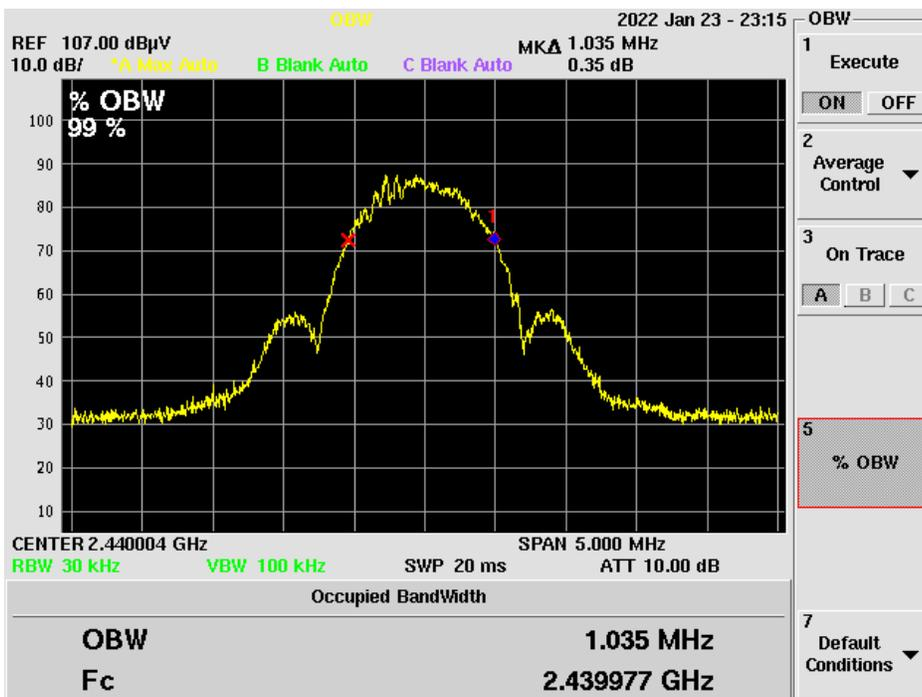
Figure 11. 99% Occupied Bandwidth Mid Channel PHY1
