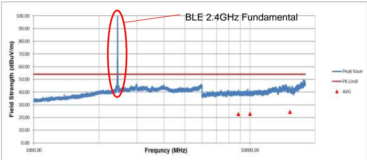
Figure 19. Unintentional Radiated Emissions, 1000 MHz – 18000 MHz (Vertical)
