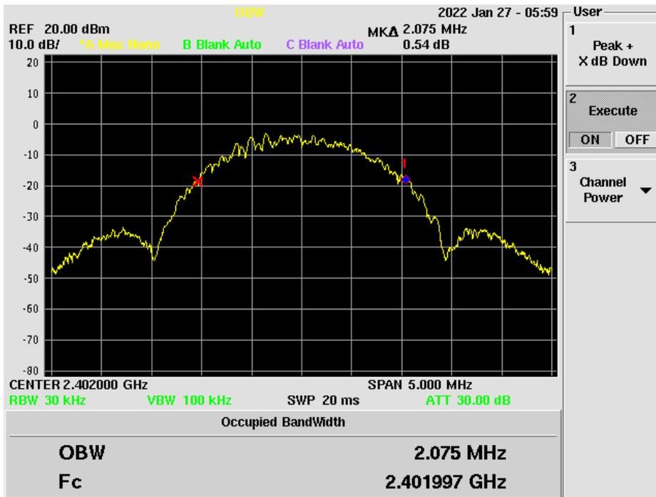
Figure 13. 99% Occupied Bandwidth Low Channel PHY2
