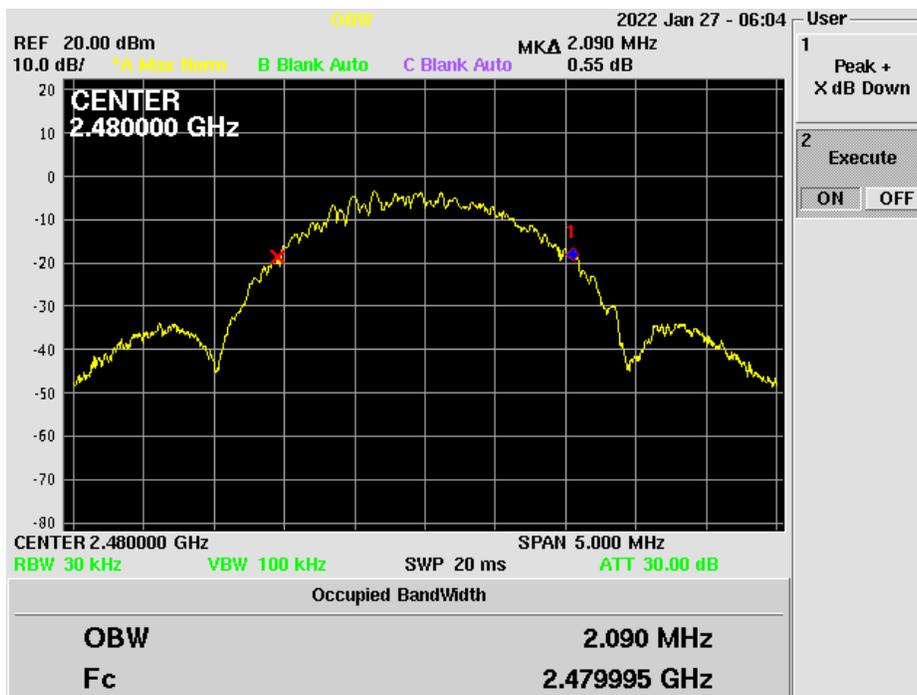
Figure 15. 99% Occupied Bandwidth High Channel PHY2
