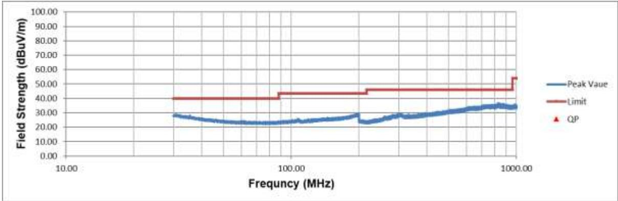
Figure 16. Unintentional Radiated Emissions, 30 MHz – 1000 MHz (Horizontal)
