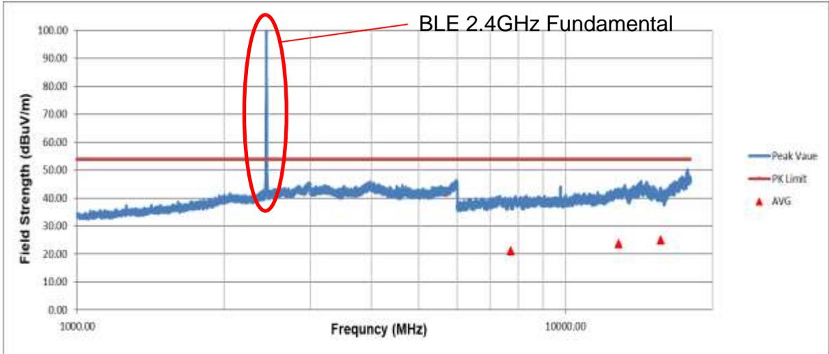
Figure 18. Unintentional Radiated Emissions, 1000 MHz – 18000 MHz (Horizontal)
