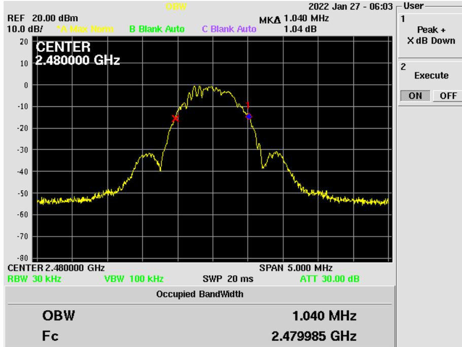
Figure 12. 99% Occupied Bandwidth High Channel PHY1
