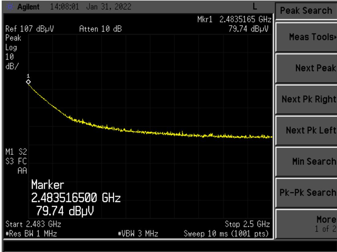
Figure 8. Radiated Restricted Band 2483.5 MHz to 2500 MHz PHY1, Peak
