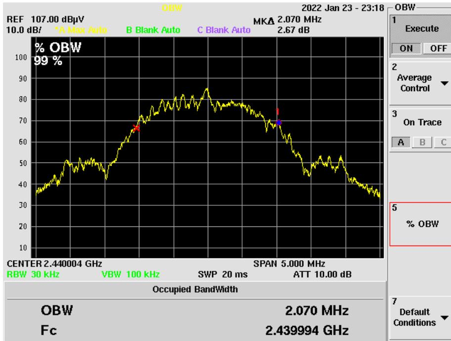
Figure 14. 99% Occupied Bandwidth Mid Channel PHY2
