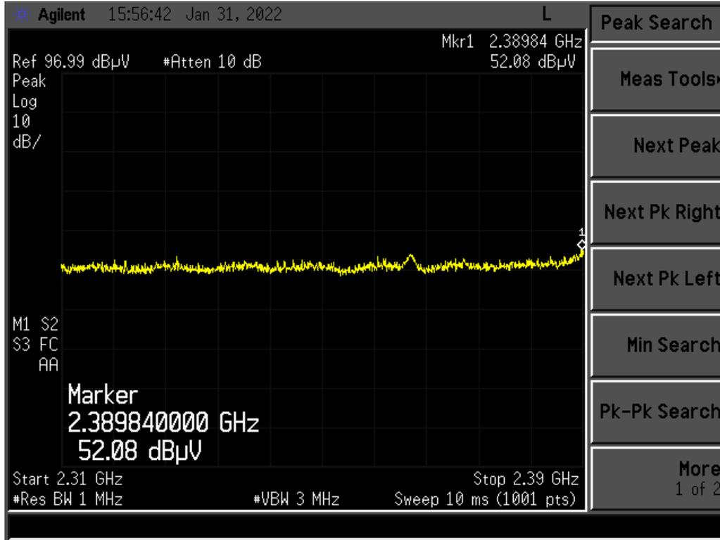
Figure 4. Radiated Restricted Band 2310 MHz to 2390 MHz PHY1, Peak
