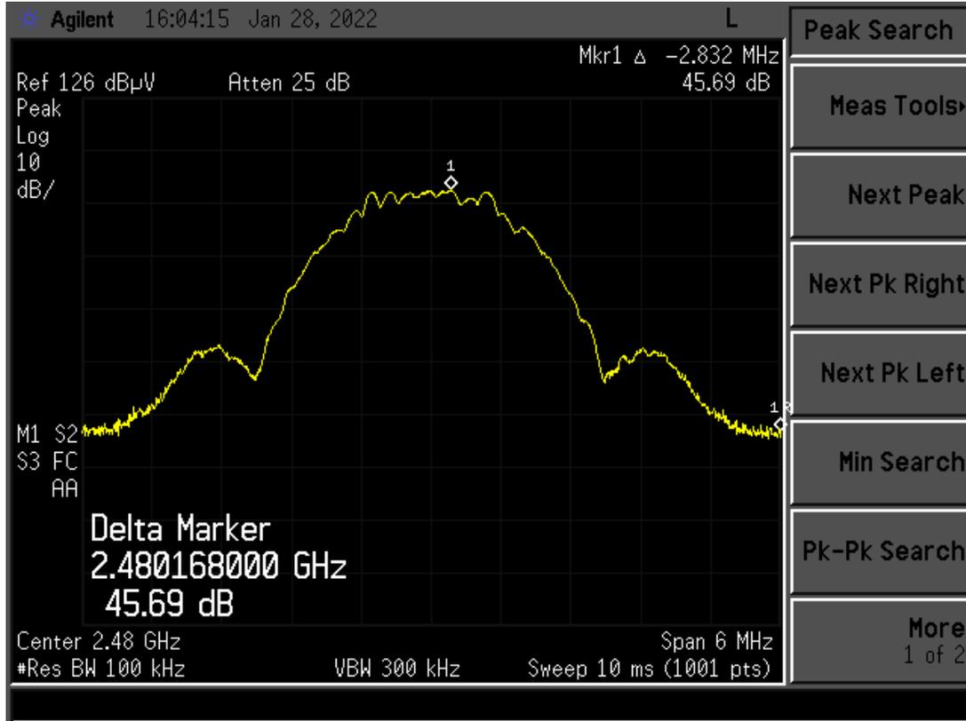
Figure 7. Band Edge Compliance, High Channel PHY2 Delta, Peak
