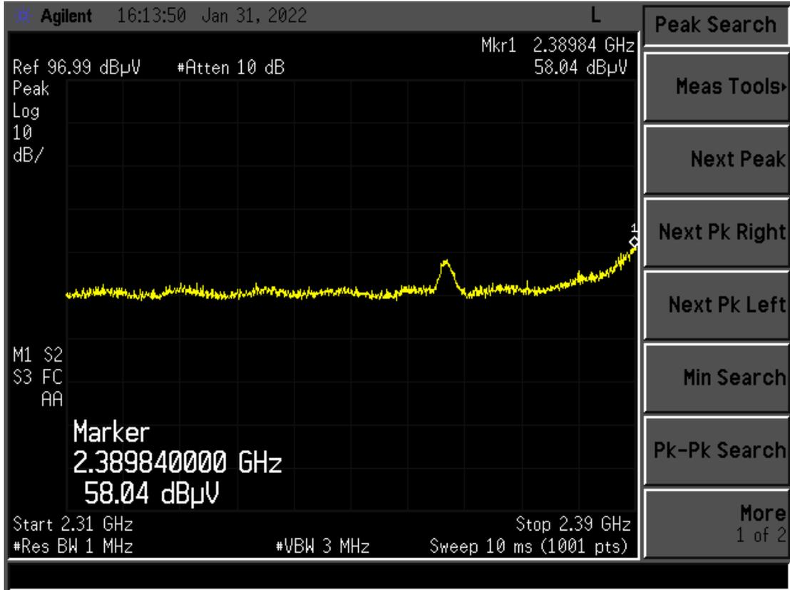
Figure 5. Radiated Restricted Band 2310 MHz to 2390 MHz PHY2, Peak
