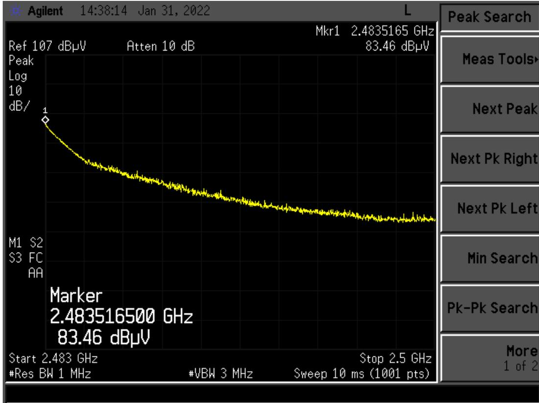
Figure 9. Radiated Restricted Band 2483.5 MHz to 2500 MHz PHY2, Peak
