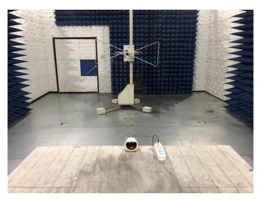
FCC RADIATED EMISSION TEST SETUP ABOVE 1GHZ
