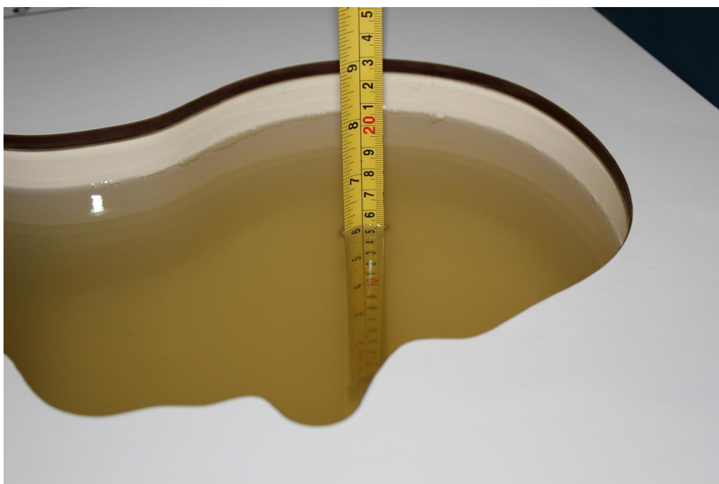
Picture 7-6: Liquid depth in the Head Phantom(2550MHz)
