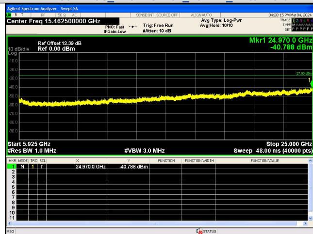
Spurious Emission:5925~25000.0 MHz IEEE 802.11ac_Channel 151_40MHz_Antenna 0
