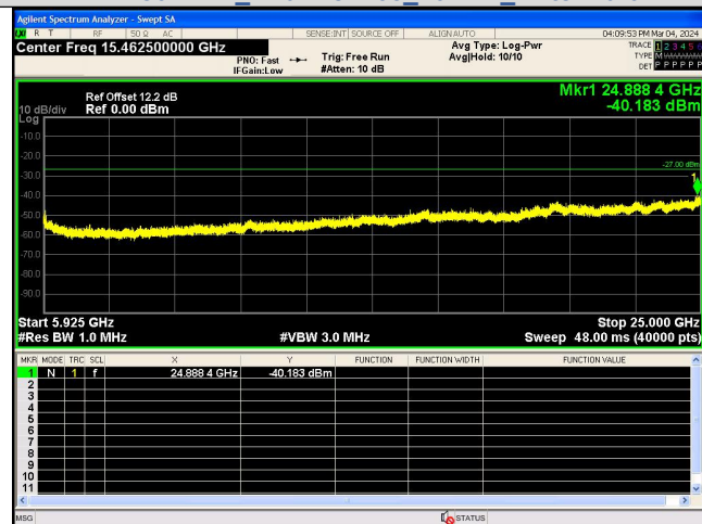
Spurious Emission:5925~25000.0 MHz IEEE 802.11n_Channel 165_20MHz_Antenna 0
