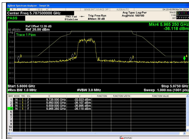
Out Of Band Emission IEEE 802.11ac_Channel 151_40MHz_Antenna 0
