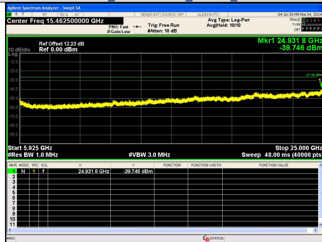
Spurious Emission:5925~25000.0 MHz IEEE 802.11n_Channel 159_40MHz_Antenna 0
