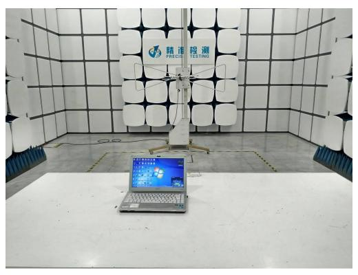
RADIATED EMISSION TEST SETUP ABOVE 1GHz
