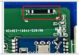
The antenna is Chip antenna.
