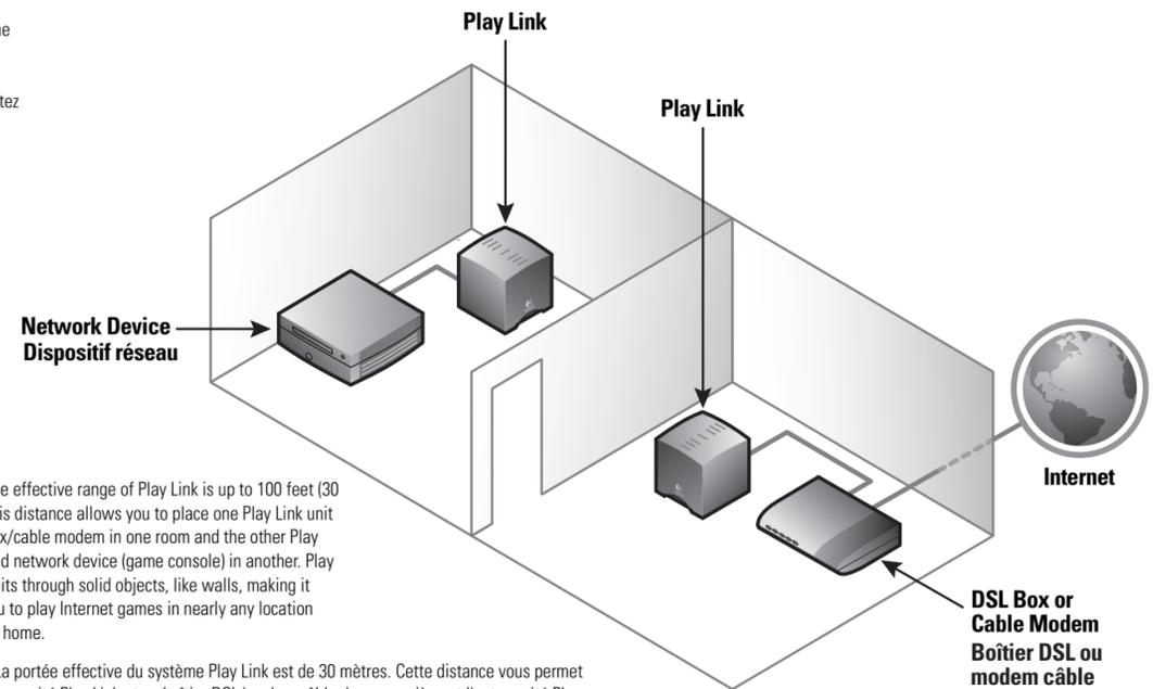
**ENGLISH** The effective range of Play Link is up to 100 feet (30 meters). This distance allows you to place one Play Link unit and DSL box/cable modem in one room and the other Play Link unit and network device (game console) in another. Play Link transmits through solid objects, like walls, making it easy for you to play Internet games in nearly any location within your home.
