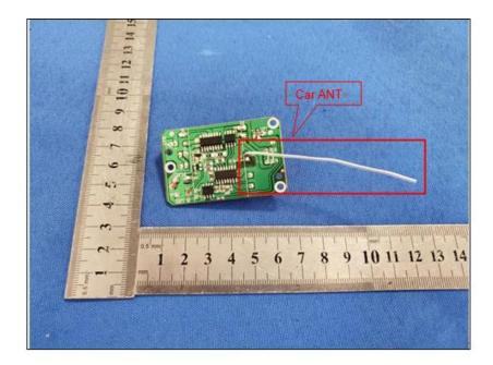
Length: 8cm Antenna Type: Wire Antenna Antenna Gain: 0dBi
