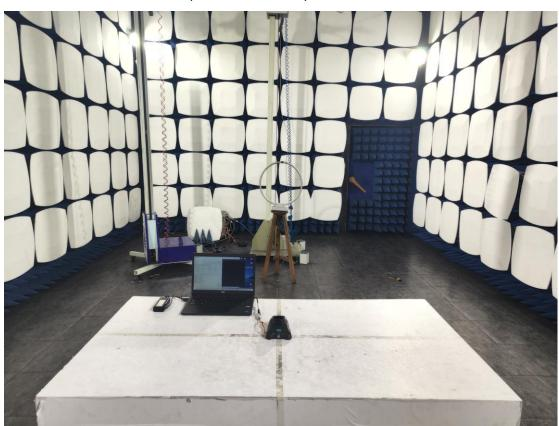
3. Radiated emission (9KHz-30MHz)
