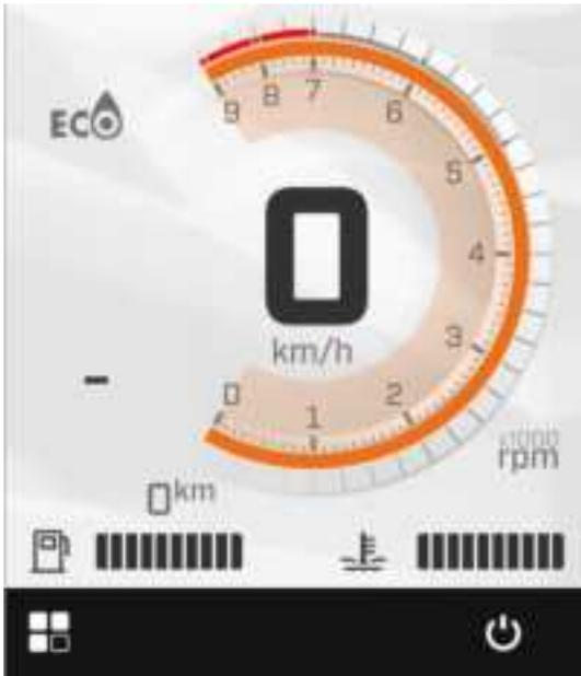
The fuel level is graphically displayed on the bottom-left side of the display. When the fuel level is low, the color will change to Red.
