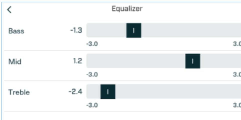
Equalizer allows the setting of the Bass, Mid and Treble ranges. Touch the area on the scale to which you wish the setting to be. Touch the back arrow to return to Audio Settings.
