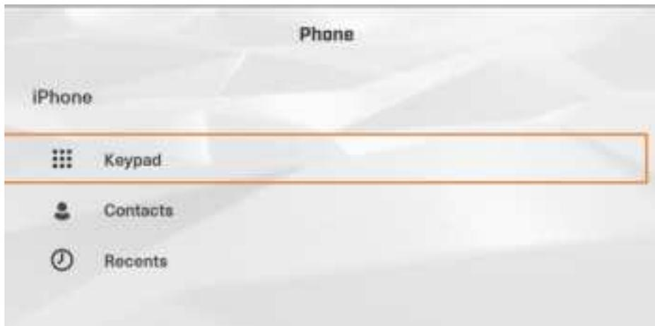
To make a call, ensure that you have connected a Bluetooth-enabled phone and headset to the Caribou display. Select Keypad and manually enter the number or select from your recent calls or Contacts lists. Touch the green phone button to initiate the call.
