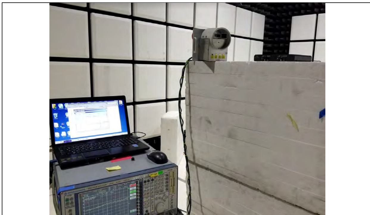
Radiated Spurious Emissions Test Configuration 18GHz – 26.5GHz
