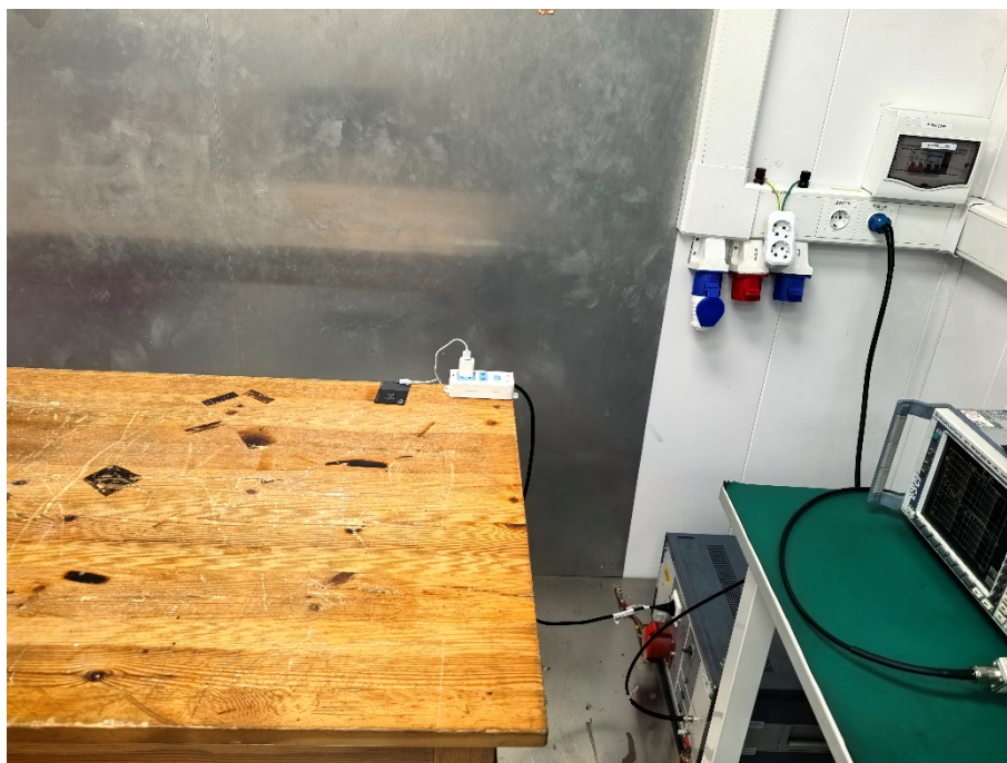
Conducted Emission at AC power line(BLE)
