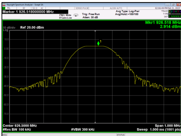
Peak output Power plot on channel 103 (1Mbps)
