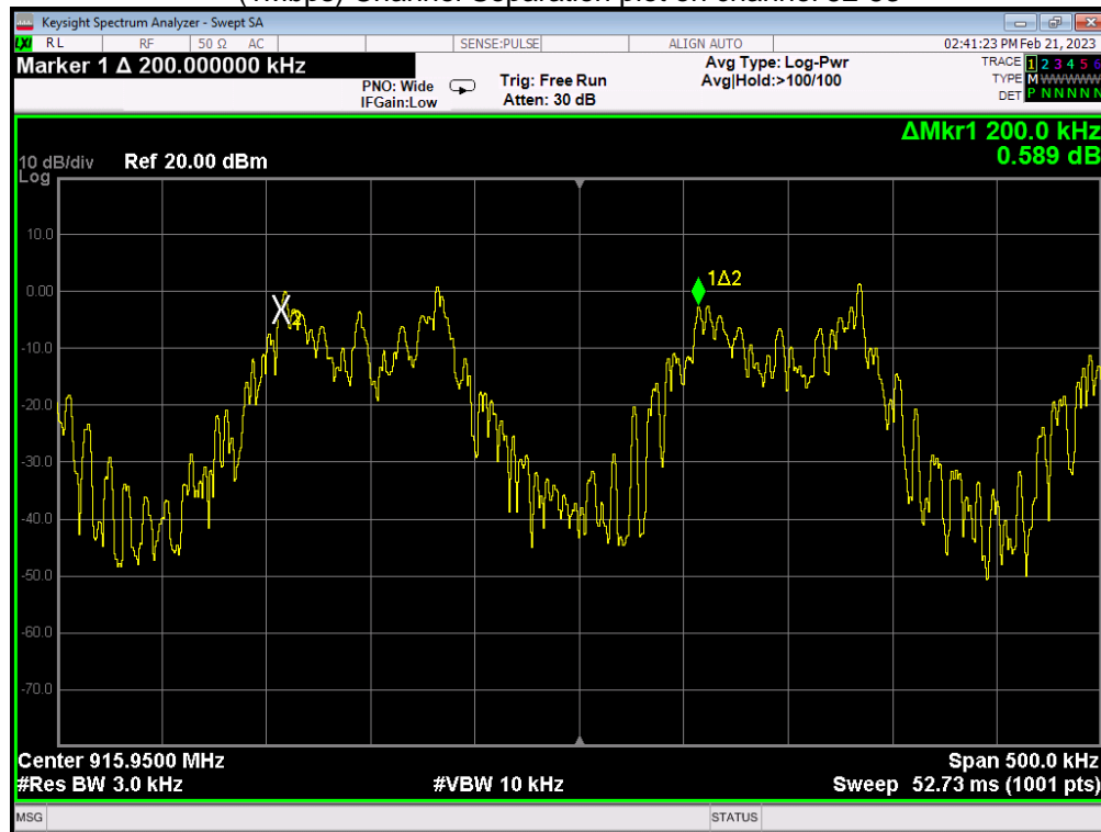
(1Mbps) Channel Separation plot on channel 102-103
