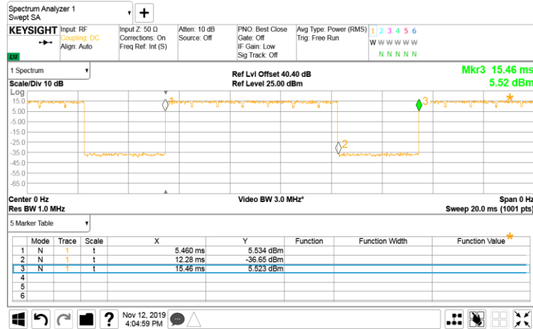
Plot 7.1.25 Transmission pulse duration and pulse period
