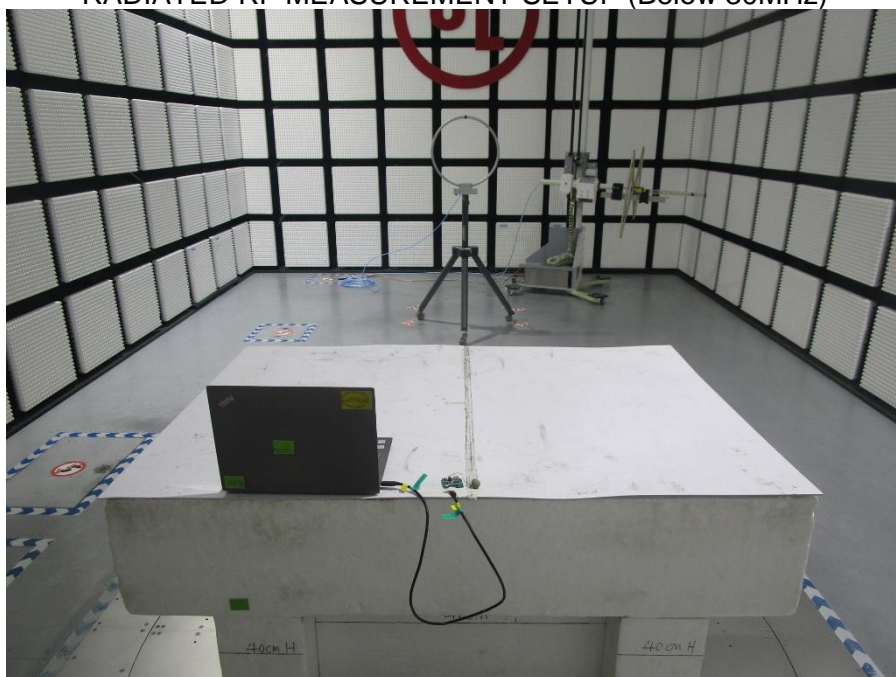
RADIATED RF MEASUREMENT SETUP (Below 30MHz)
