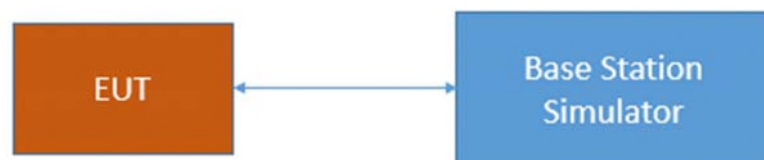
Test Setup FCC Part 22/24/27/90 Cellular; Frequency stability
