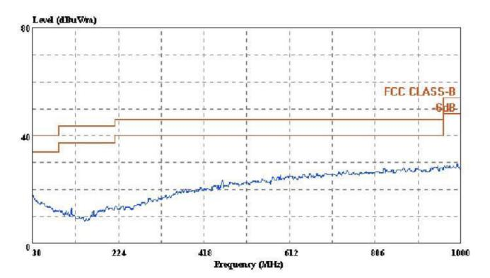
Condition: FCC CLASS-B 3m ATC VULB9163(NEW) HORIZONTAL
