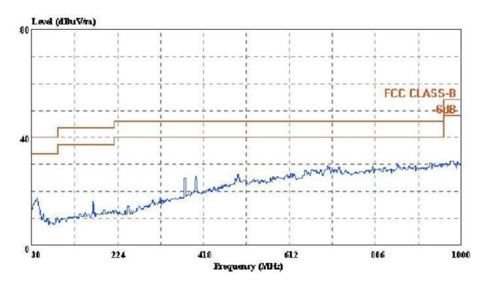
Condition: FCC CLASS-B 3m ATC VULB9163 (NEW) VERTICAL
