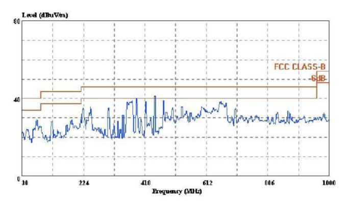
Condition: FCC CLASS-B 3m ATC VULB9163(NEW) HORIZONTAL
