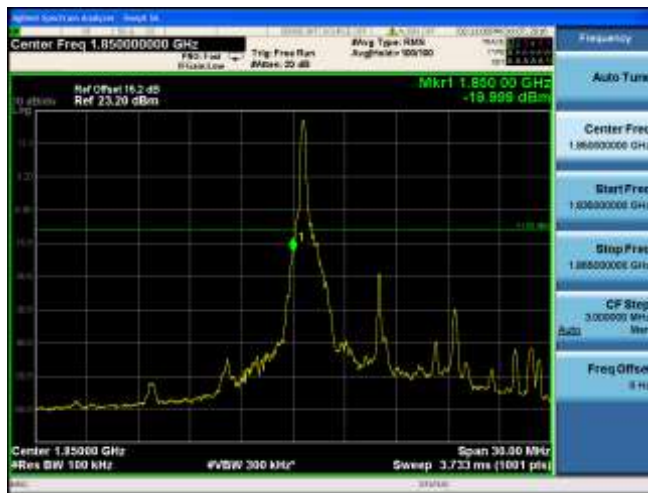
CH18675 (1857.5MHz) QPSK Bandwidth 15MHz 1RB#0
