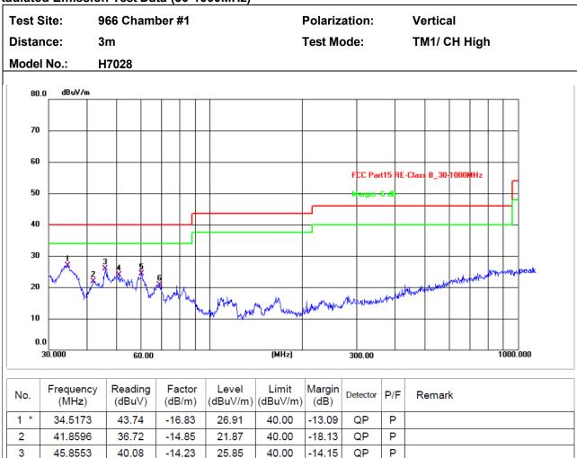
Note: Level = Reading + Factor Margin = Level - Limit
