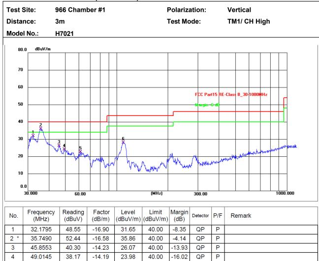
Note: Level = Reading + Factor Margin = Level - Limit
