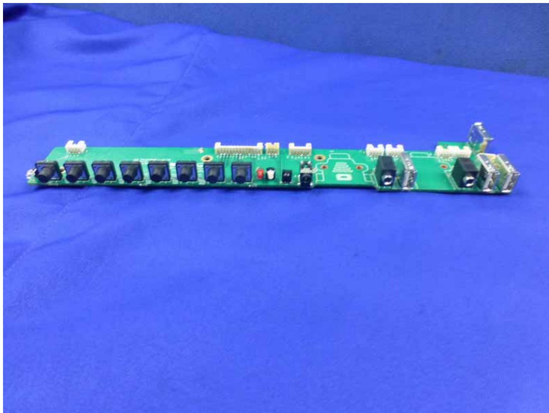
Figure 19 I/O Port of the Control Board
