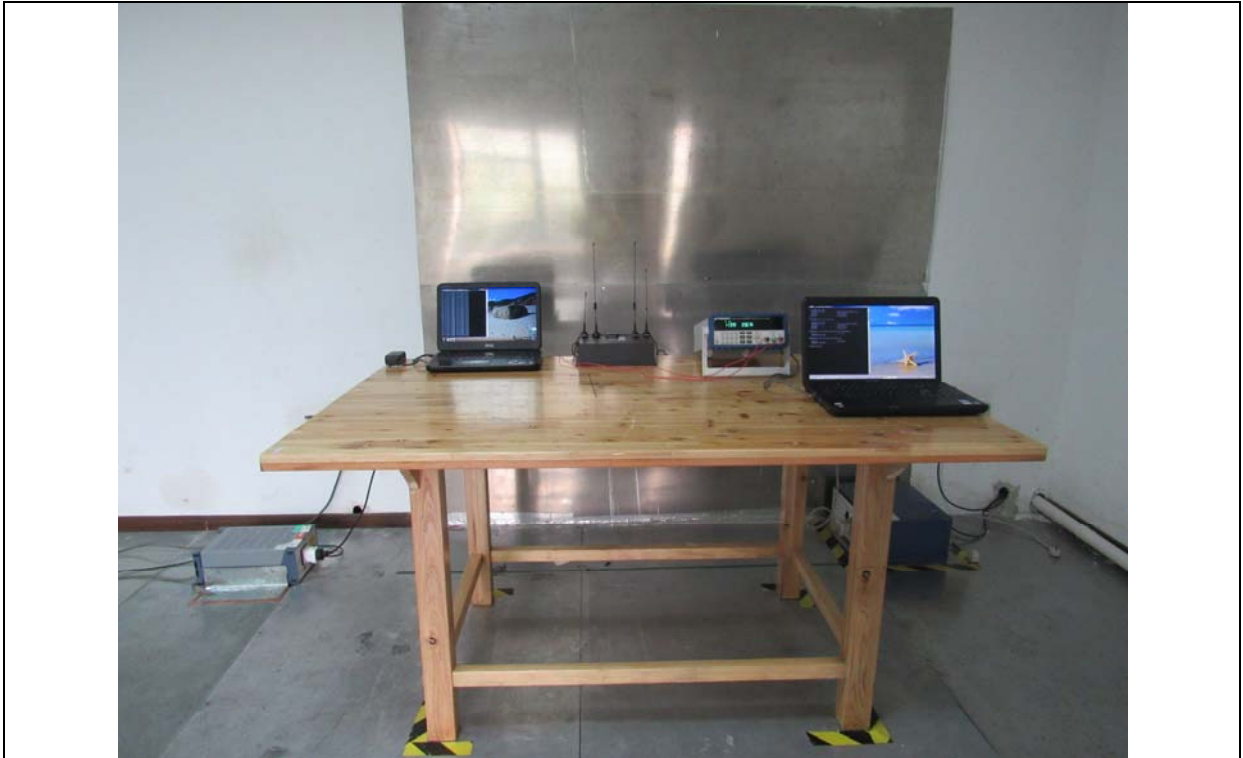
Conducted Emissions Setup Front View
