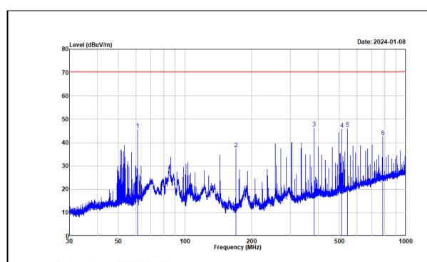
Project No. : RWA0202400009 Test Mode : Microwave Test Voltage : AC 120V/60Hz
