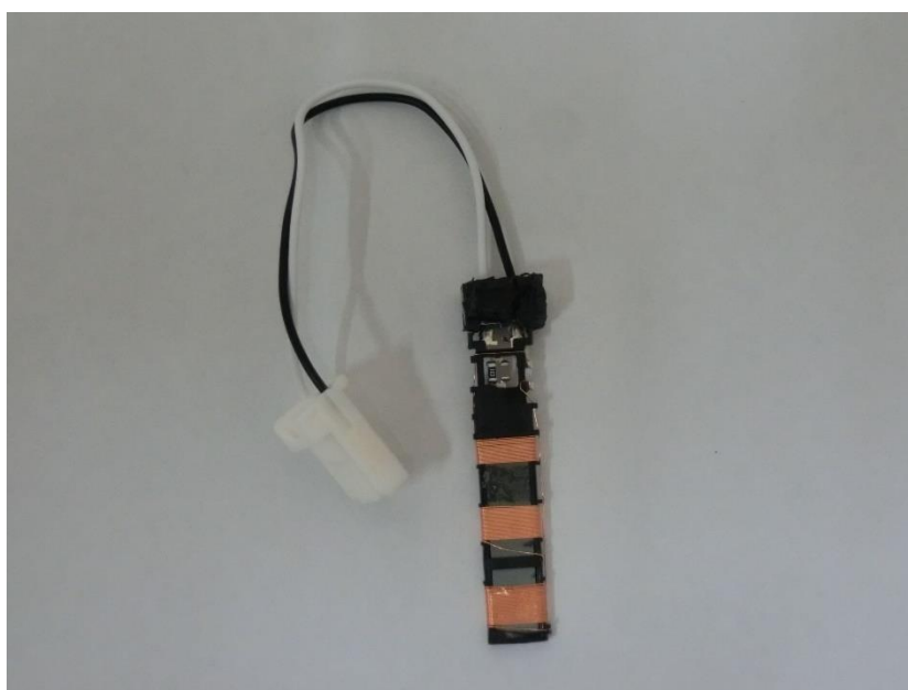
Figure 8.16 LF-antenna InF,InR,TG internal (back view)
