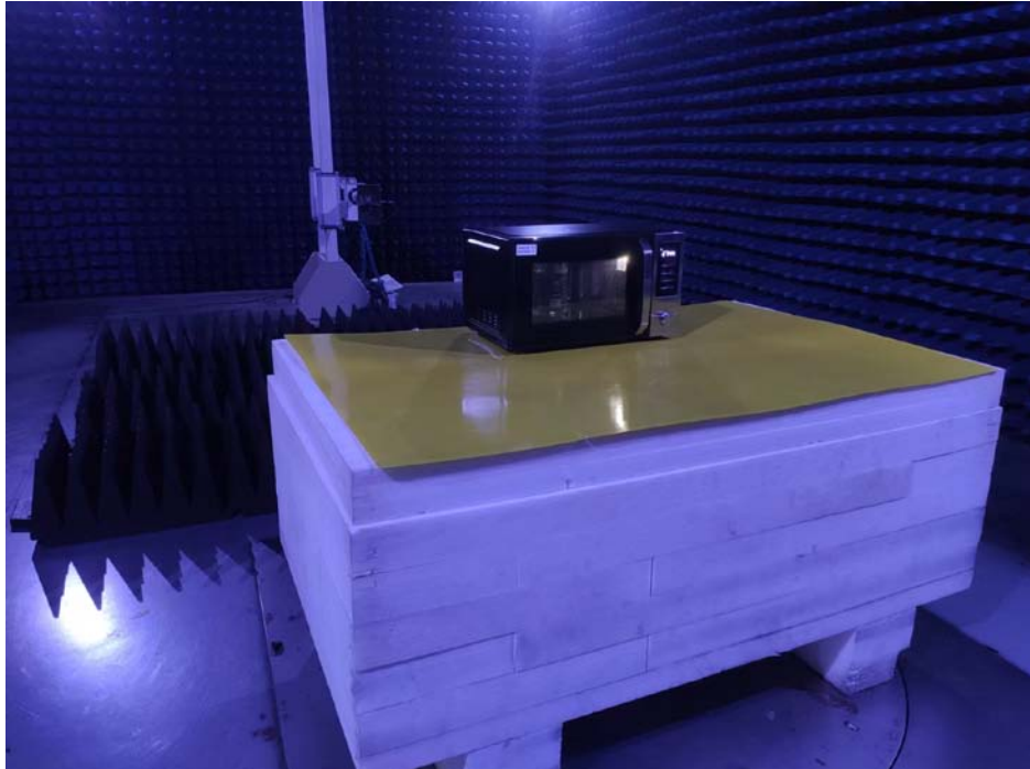
Photo of Radiation Emission Measurement- Above 1GHz
