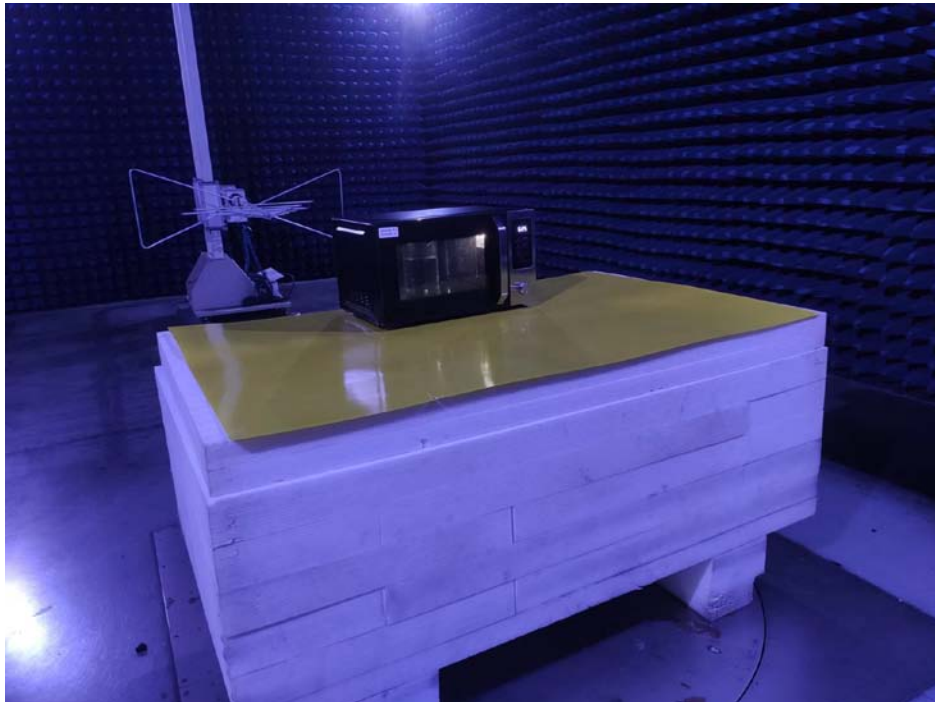
Photo of Radiation Emission Measurement- Above 1GHz
