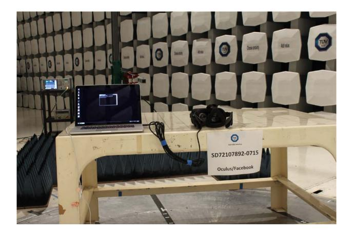
Radiated Emissions Test Setup (above 1GHz)
