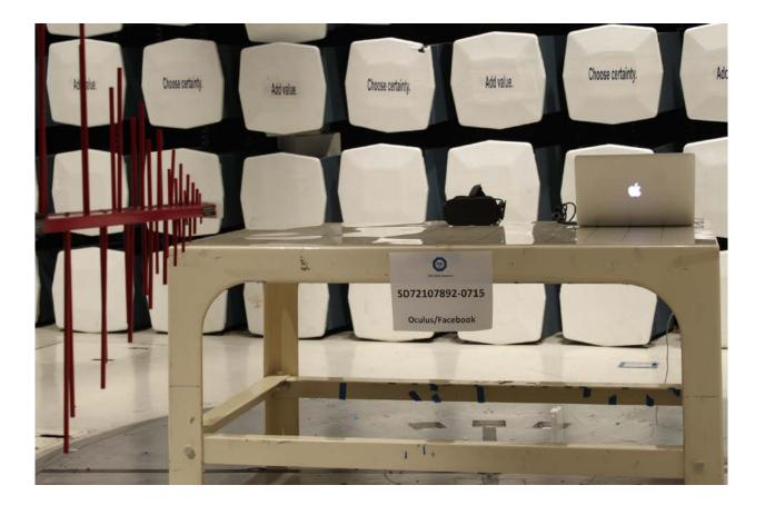
Radiated Emissions Test Setup (below 1GHz)
