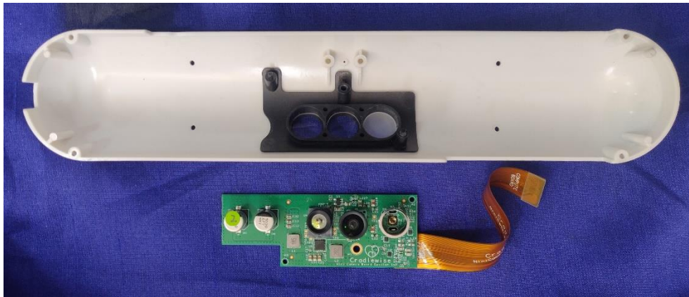
Photo 15: Monitor cover and camera board
