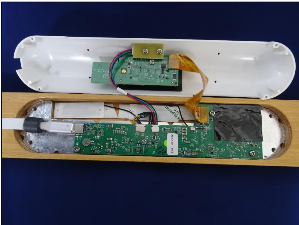
Photo 14: Monitor arc with monitor cover open
