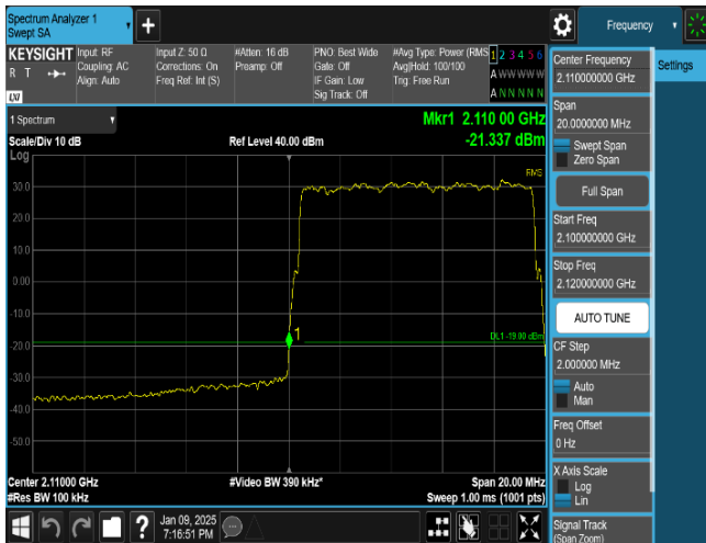
Plot 8-47. Band Edge Emission Summary Data Plot (LTE_B66_1C_10M_16QAM - Low Edge, Port 0)
