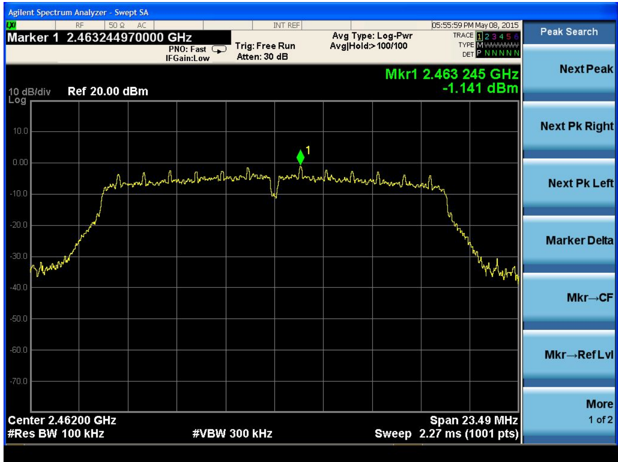
(Plot 4.4.2 C: Channel 11: 2462MHz @ 802.11g)
