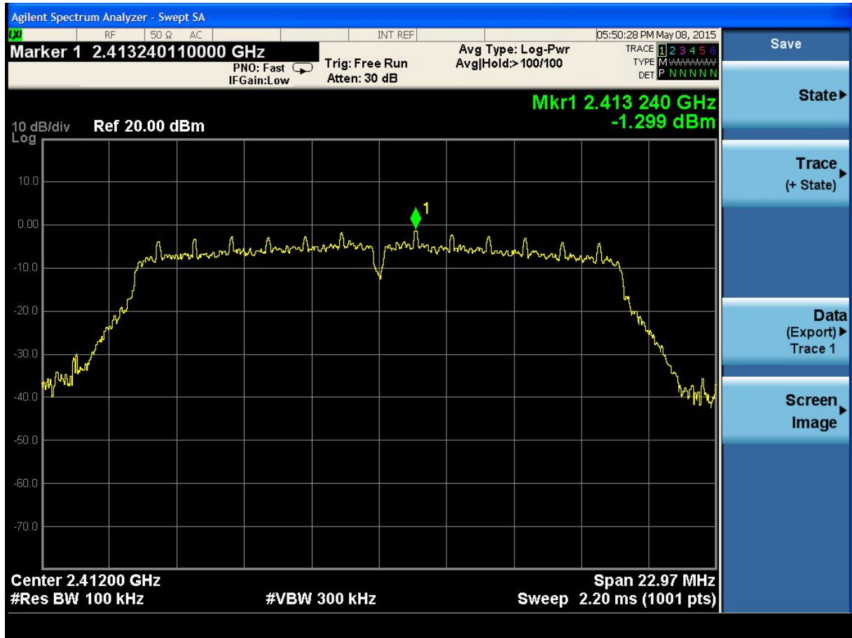
(Plot 4.4.2 A: Channel 1: 2412MHz @ 802.11g)
