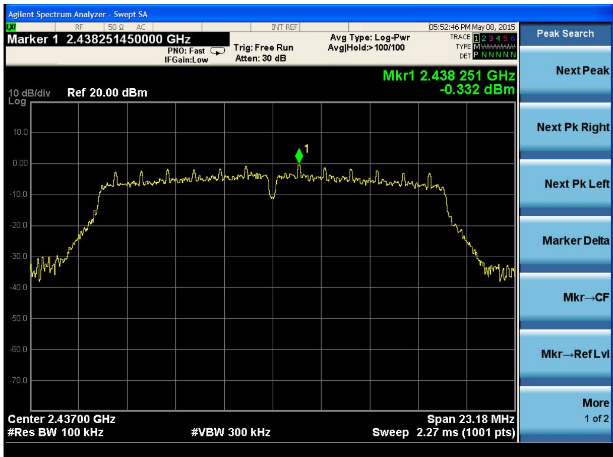
(Plot 4.4.2 B: Channel 6: 2437MHz @ 802.11g)
