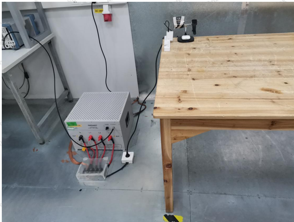
Photo of Conducted Emission Measurement
