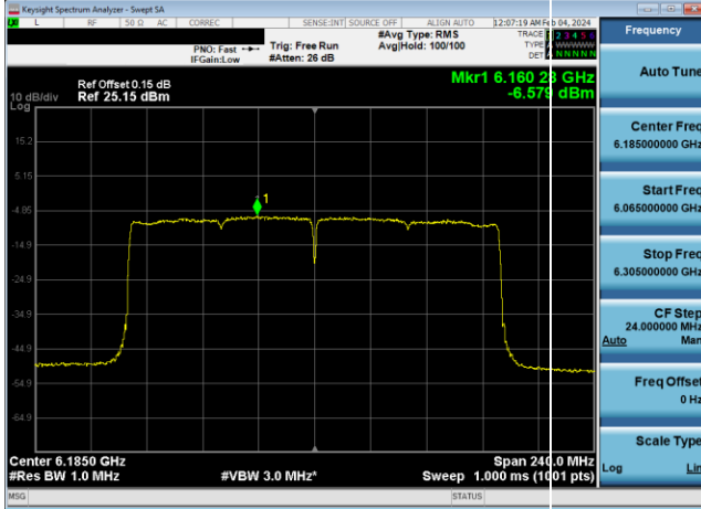
Plot 7-602. Power Spectral Density Plot SDM Diversity Antenna WF8 LPI (160MHz 802.11ax (UNII Band 5) – Ch. 47, MCS2)
