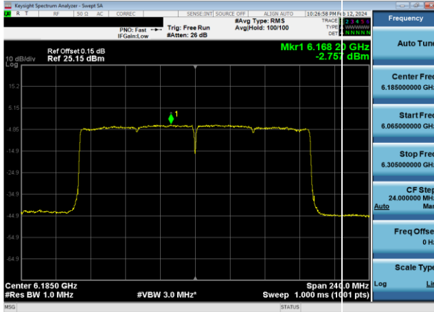
Plot 7-554. Power Spectral Density Plot CDD Primary Antenna WF5B Standard Power (160MHz 802.11ax (UNII Band 5) – Ch. 47, MCS2)
