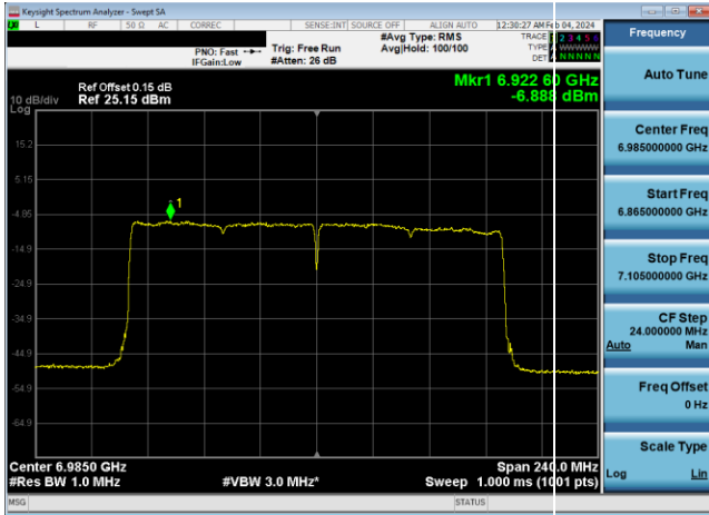
Plot 7-626. Power Spectral Density Plot SDM Diversity Antenna WF8 LPI (160MHz 802.11ax (UNII Band 8) – Ch. 207, MCS2)
