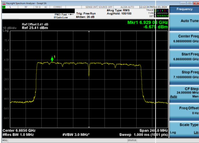
Plot 7-546. Power Spectral Density Plot SDM Primary Antenna WF5B LPI (160MHz 802.11ax (UNII Band 8) – Ch. 207, MCS11)
