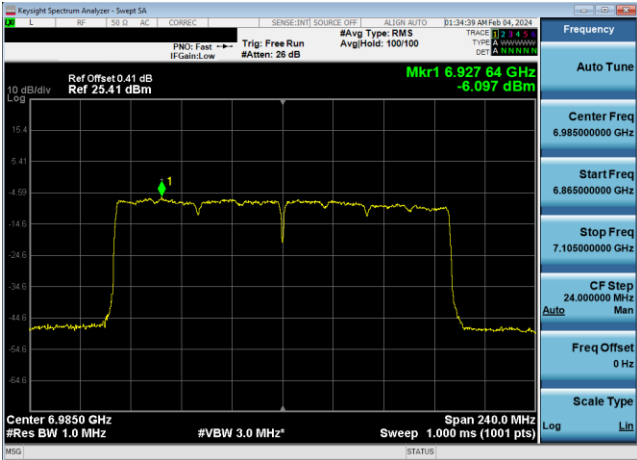
Plot 7-547. Power Spectral Density Plot SDM Primary Antenna WF8 LPI (160MHz 802.11ax (UNII Band 8) – Ch. 207, MCS11)
