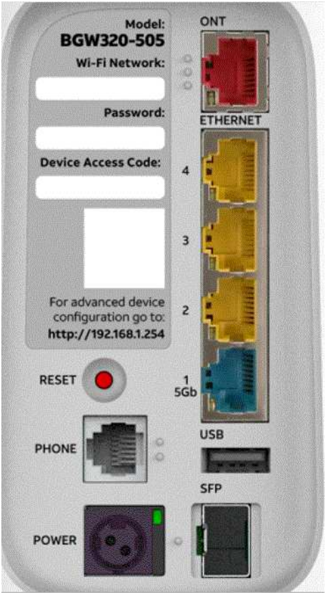
Figure 3-8 BGW320-505 Physical connections
