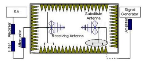
In the chamber, an substitution antenna for the frequency band of interest is placed at the reference point of the chamber. An RF Signal source for the frequency band of interest is connected to the substitution antenna with a cable that has been constructed to not interfere with the radiation pattern of the antenna. A power ( $P_{\text{Mea}}$ ) is applied to the input of the substitution antenna, and adjust the level of the signal generator output until the value of the
