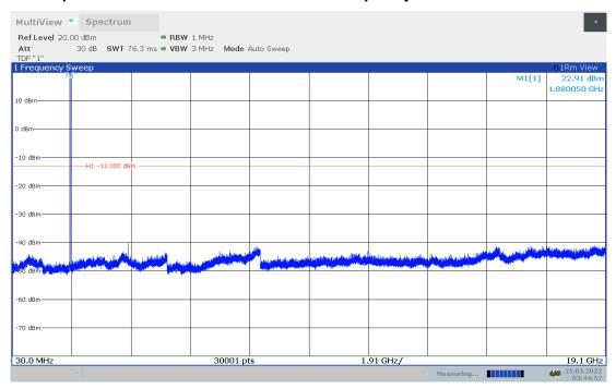
LTE band 5 : 30MHz – 8.49GHz Spurious emission limit –13dBm.
