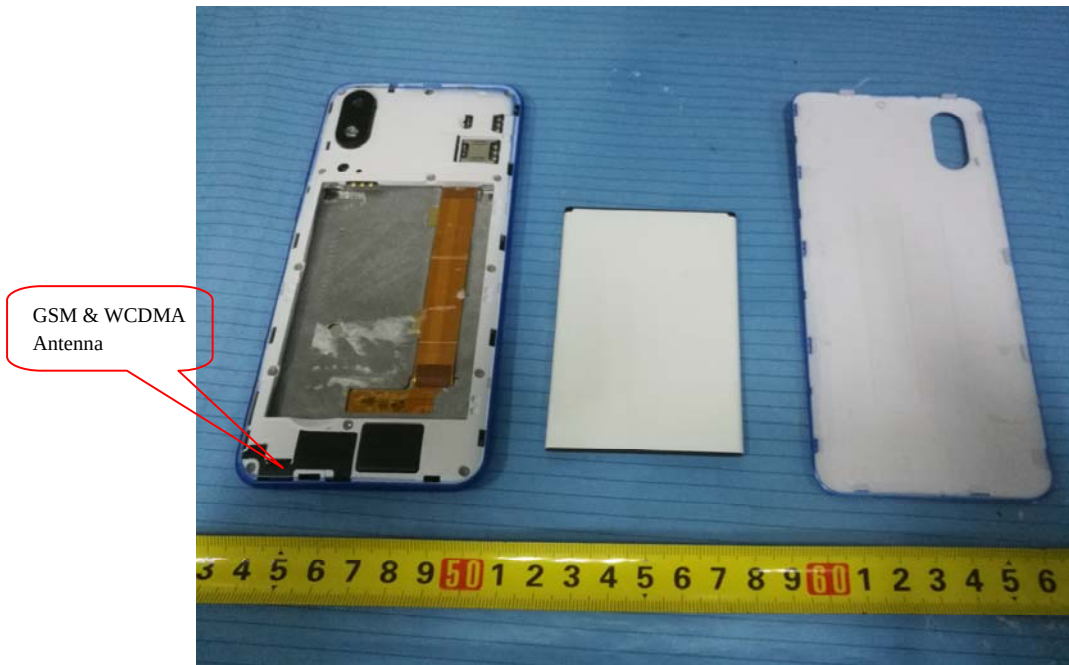
EUT – Cover off View 1
