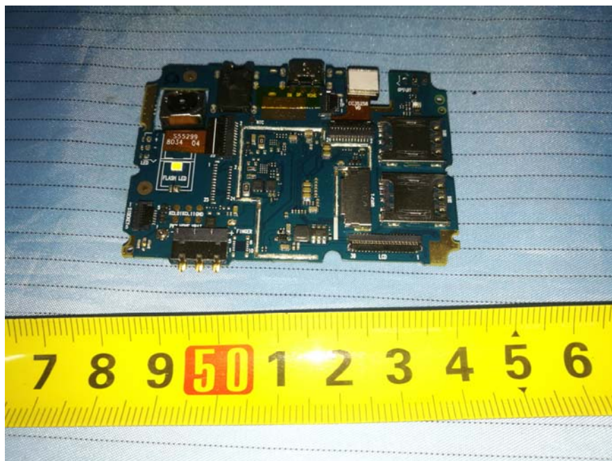
EUT – Mainboard Bottom Shielding off View
