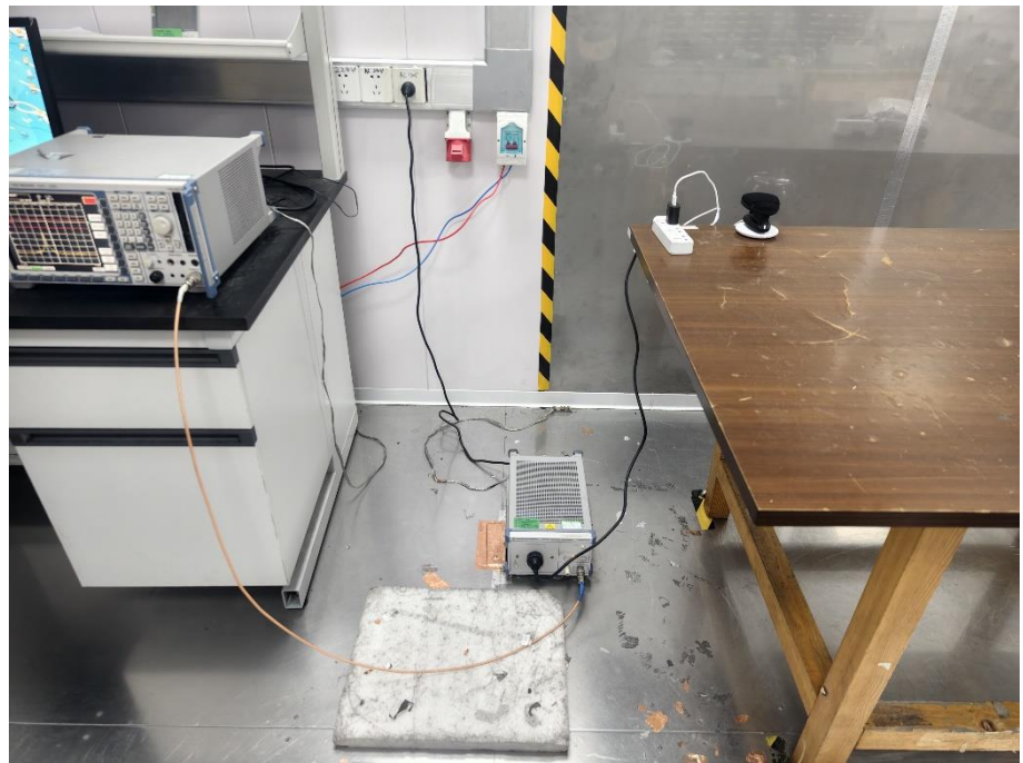
Conducted Emission Test Setup
