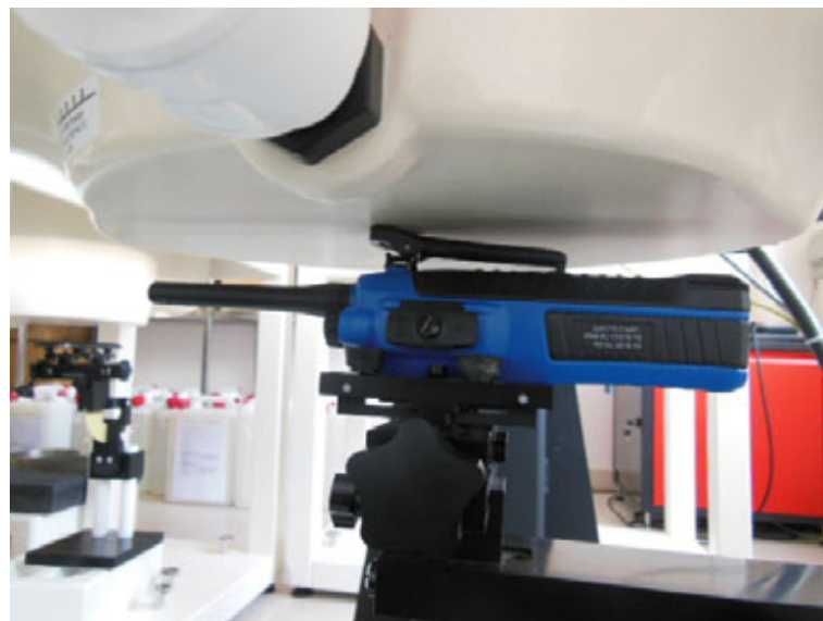
Body-worn, the front of the EUT towards ground
