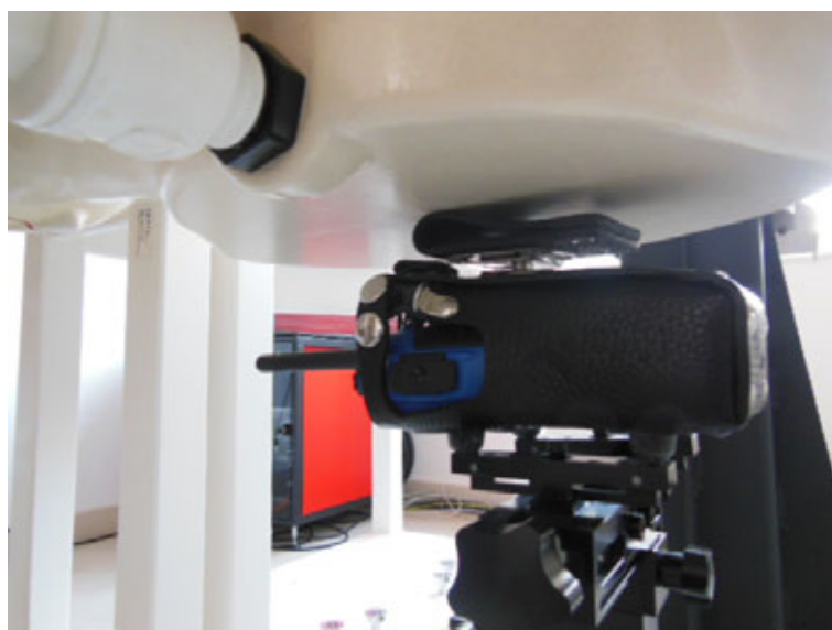
Body-worn, the front of the EUT towards ground with LC1
