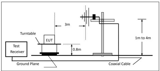
(c) For radiated emissions above 1000MHz
