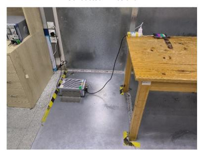
Radiated Emissions From 30MHz-1000MHz
