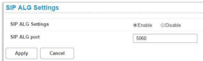
The screenshot shows a configuration window titled "SIP ALG Settings". It contains two rows of settings. The first row is "SIP ALG Settings" with two radio buttons: "Enable" (which is selected) and "Disable". The second row is "SIP ALG port" with a text input field containing the number "5060". At the bottom of the window are two buttons: "Apply" and "Cancel".
