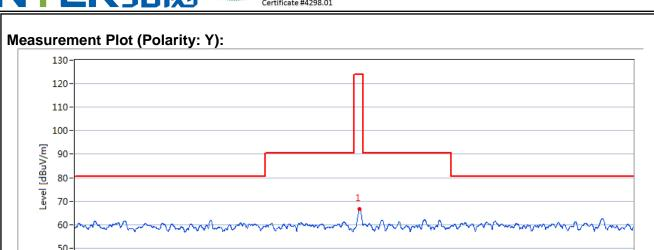
50 40 30-13.11 14.01 Frequency [MHz] **Measurement Result:** Pre-scan Level MaxPeak Limit MaxPeak Final Test Level Frequency MHz Margin dB MaxPeak dBuV/m dBuV/m dBuV/m 13.501 67.1 57.4 80.5 23.1
