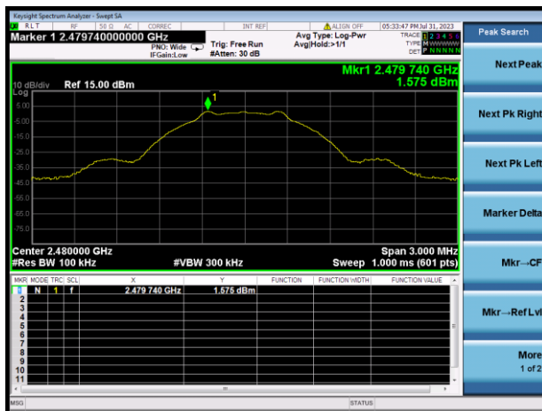
GFSK (BLE 1Mbps) HIGH CHANNEL, CARRIER LEVEL
